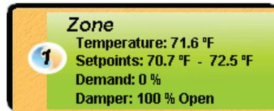
Figure 5 - Typical VAV Zone Controller icon
