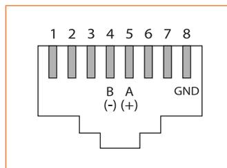
Figure 8 - Raccordement RJ45
