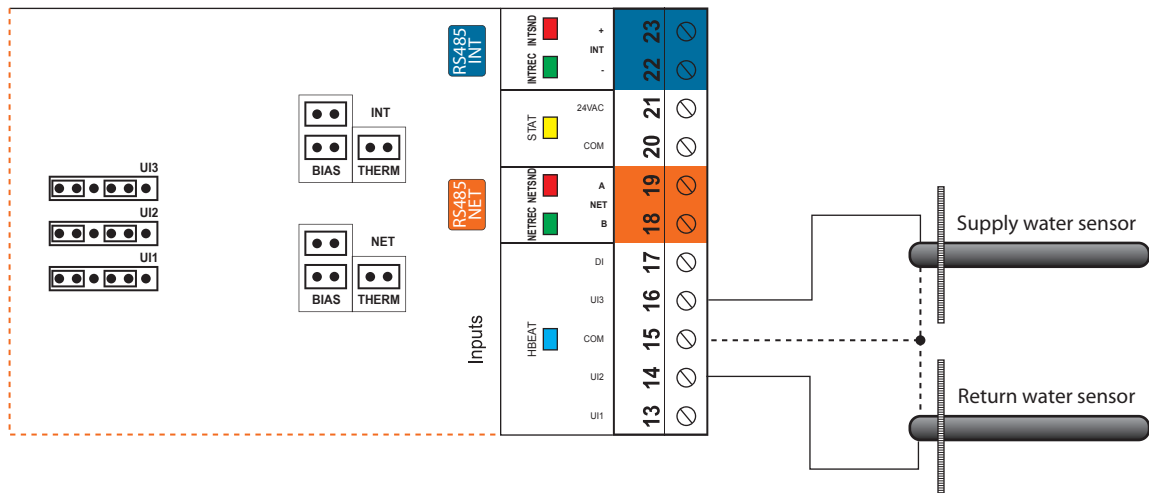
Figure 6 - Connecting the Water Temperature Sensors
