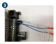
Match insulated conductors, twist together, and install under communication terminal screws. *Note*: There should never be more that 2 communication wires installed under a single screw.
