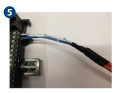
Secure and insulate exposed shield wires to avoid accidental grounding.
