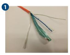
Strip only the outer jacket back 2", taking care to not damage the wires inside.
