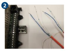
Remove foil and support filament (when applicable), separate all wires, and strip individual insulated conductors.
