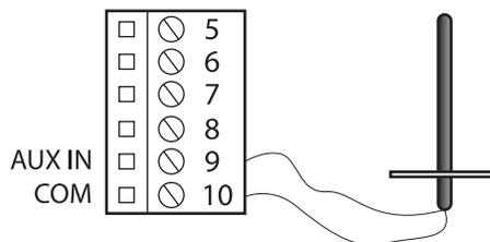
Figure 5 - Connecting the Auxiliary Input
