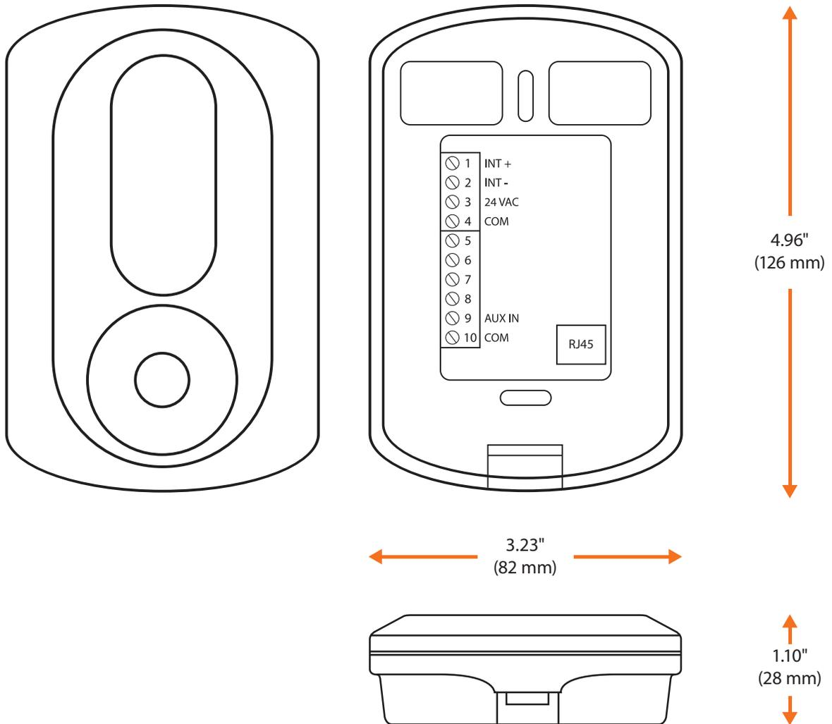
Figure 9 - T1000 Size Diagram
