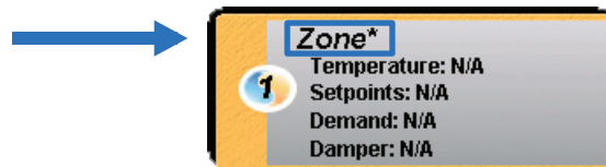
Figure 15 - Offline Modification Marker
