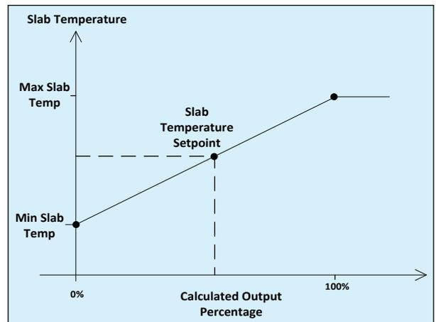
Figure 28 - Slab target scale
