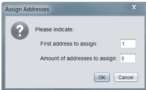
In the example image above, addresses 1 through 5 will be assigned to five VC2000s. If address 3 has already been assigned to another controller somewhere on the network, then addresses 1 through 6 will be assigned instead, skipping over address 3. Addresses can be reassigned later using the Focus's Address Management feature.
