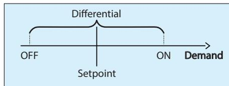
Figure 26 - Differential diagram
