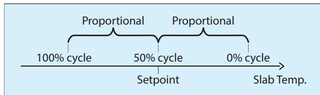
**Figure 29 - Radiant Floor proportional band**
