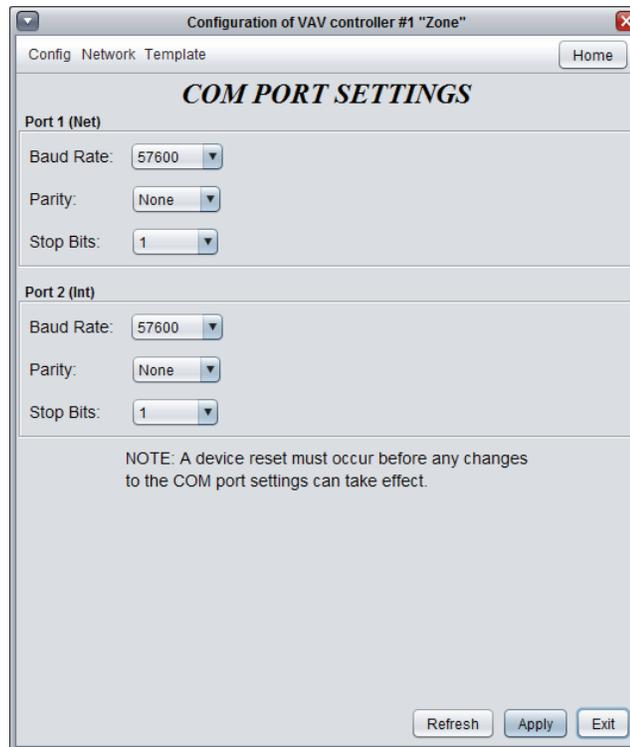
Figure 42 - COM Port configuration screen
