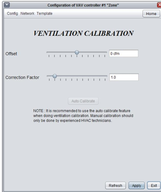
Figure 33 - Ventilation Calibration configuration screen
