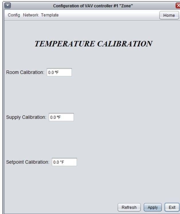
Figure 32 - Temperature Calibration configuration screen
