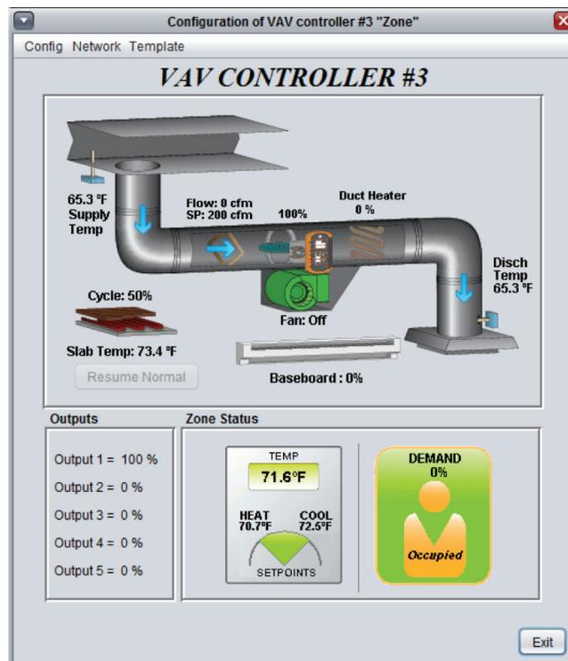
Figure 11 - VAV Zone Controller home screen
