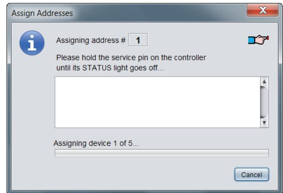
Only the controller whose SERVICE button is held down will receive the assigned address, so you must physically go to the appropriate controller and hold down the SERVICE button until the Status Light goes off (indicates that the address has been assigned). It should not take more than five seconds to receive the address once you begin holding the button.
