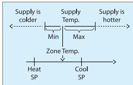
**Figure 23 - Supply temperature deadband**
