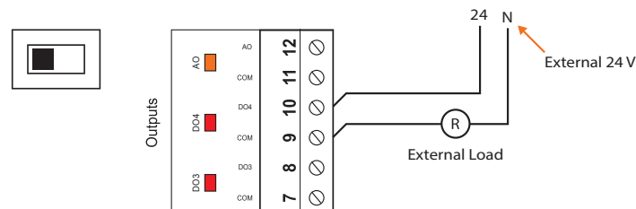
Figure 12 - Connection of Passive Output 3 and 4
