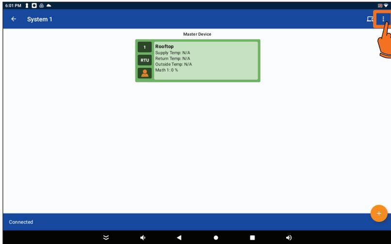
1. It is possible to address the VC2000 zone controllers directly from the display. From the System page, tap on the configuration icon.
