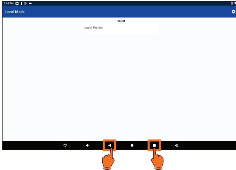
1. Upon start-up of the Focus app, the user can choose whether or not to pin the app (a pinned app cannot be exited without unpinning it). To unpin the app, hold the ◀ and the ■ icons at the same time to unpin the Focus App and return to normal navigating mode of the display.
