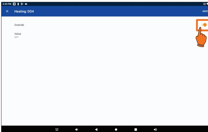
2. Enable the override by sliding the override slider icon.
